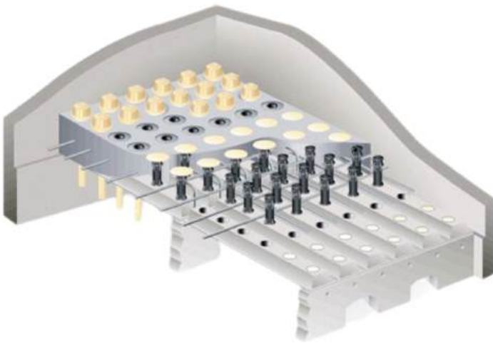
monolithic corrugated panel filter floor
